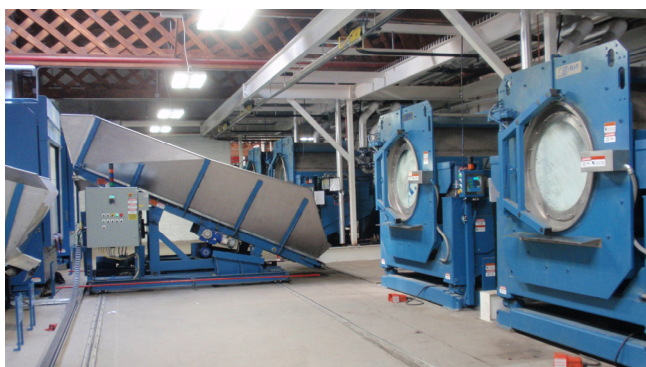
New washing machines have decreased Roscoe's use of city water from 280,000 gallons to 180,000 gallons per week: more than a 35 percent reduction.
